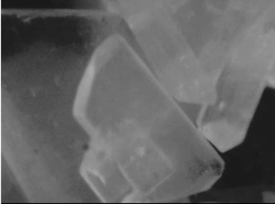
FIGURE 10.12 Photograph of recovered struvite crystals from an anaerobic digester at Durham Advanced Wastewater Treatment Plant, Tigard, Oregon (200× magnified).
